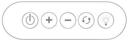
Press once to turn blower and lights ON. When button is pressed, the blower speed increases gradually for 5 seconds before it returning to default setting. "+", "-" and "mode buttons are disabled during start up. Press a second time to turn blower OFF. Blower times out automatically after 20 minutes.
